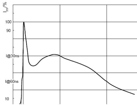
ESD pulse waveform according to IEC61000-4-2
