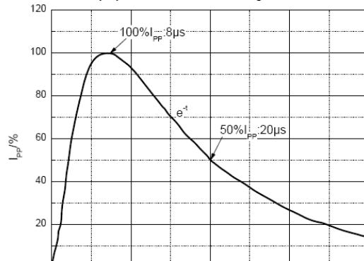
8/20μs pulse waveform according to IEC 61000-4-5
